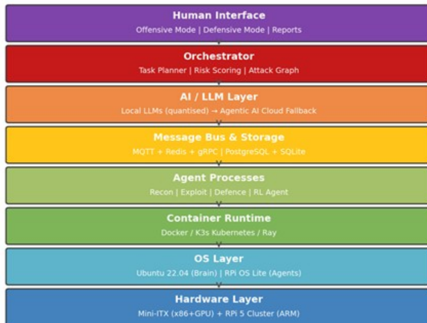
Figure 2: PenBox-DMAS Software Stack — Eight-layer architecture from hardware through OS, containers, agent processes, message bus, AI/LLM layer, orchestrator, to human interface.
